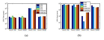
Fig. 2: Results for single guest domain: (a) CPU time per execution and (b) Execution count per second.
