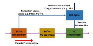
Fig. 3. The architecture of TCon.
