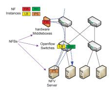
Fig. 1: Service Chain Example:  $FW \to LB \to IPS \to Monitor$
